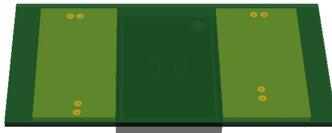
Figure 5.4 Recommended PCB Layout — Bottom Layer
